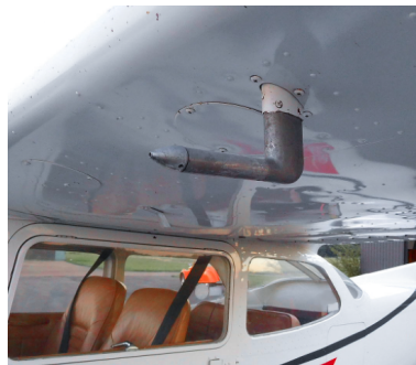
Figure 2: Pitot tube on a wing of small plane
