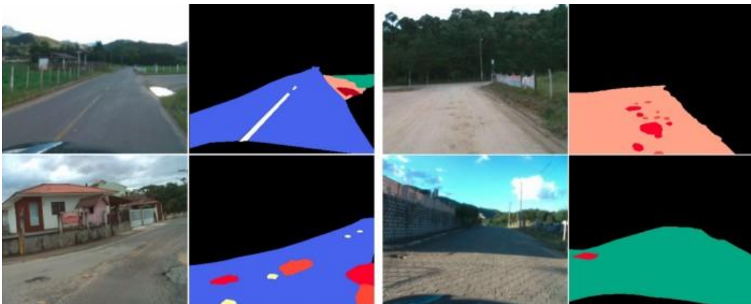
Figure 4. Pairs of images specifying input image and classified that are used for validation [7]
