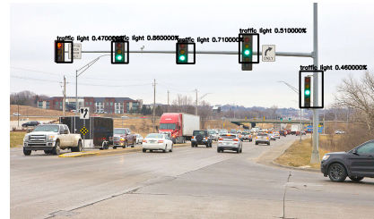
(b) traffic lights detected by second model iteration
