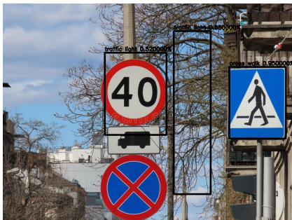
(c) traffic signs detected by first model iteration
