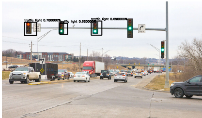
(a) traffic lights detected by first model iteration
