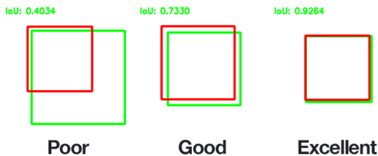
Figure 2: An example of computing Intersection over Unions for various bounding boxes An evaluation of the Intersection over Union for the custom object detection has been presented further in the document.
