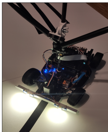
Figure 16 – Robot following line with lights turned on. The idea of mounting lights was to use them to illuminate the track in case of poor lighting conditions. This idea was not developed because the mounted lighting generated point light that interfered with the image processing algorithm.
