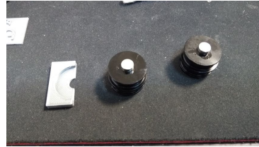
Figure 4: Picture of designed centering tool after mounting the magnets
