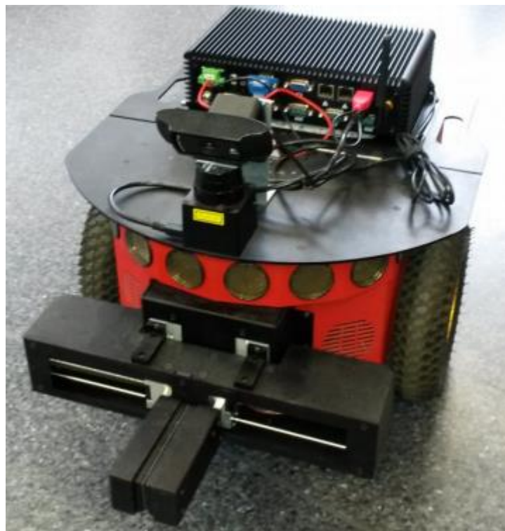
Figure 1 - Pioneer 3DX robot used
