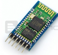
Figure 4: HC-05 bluetooth module
