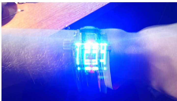
Figure 2: Displaying "1234" number by POV
