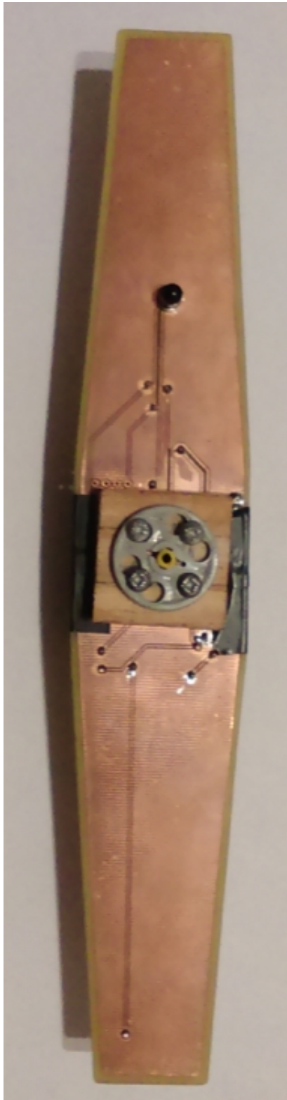
(a) bottom layer, wooden block and small hole for a shaft of DC motor
