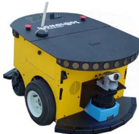
Figure 8. PowerBot™ carries over 100 kg of payload.
