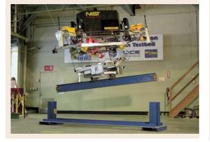
**Table 47.6** (c) Teleoperated rebar placing robot [47.11]
