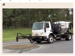
Table 47.8 Road maintenance (b) Semi-autonomous road crack sealing robot [47.69]
