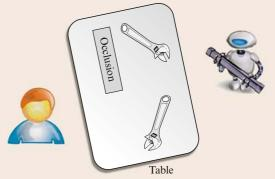
Fig. 58.13 Robonaut using visual perspective taking to disambiguate the intended referent when asked to hand me the wrench. The human can only see one wrench, but the robot can see both. The robot correctly hands the wrench that both can see
