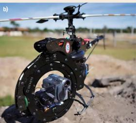
Fig. 50.1a,b Man-packable UAVs used to search portions of Mississippi during the hurricane Katrina response: (a) an anonymous fixed-wing UAV and (b) an iSENSYS IP3 rotary-wing UAV (courtesy of CRASAR)
