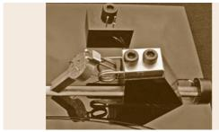
Fig. 3.18 The Elliptec piezoelectric motor
