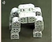
Fig. 39.1a-c Examples of self-reconfigurable robots: (a) the Polybot, a chain-based system [39.1]; (b) the Crystal, a two-dimensional lattice-based system [39.2]; (c) MTRAN [39.3], which can take on the characteristics of either type
