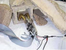
Fig. 50.8a,b Examples of legged and crawler robots. (a) Hexapod (legged) robot from the RHex project traversing a portion of the NIST test bed (courtesy of R. Sheh) and (b) Terminatorbot being tested in rescue test bed (courtesy of R. Voyles)
