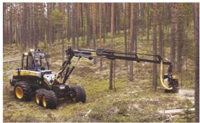
Fig. 46.1 Cut-to-length (CTL) harvester made by Ponsse Oy Ltd. [46.3]
