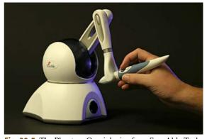
**Fig. 30.5** The Phantom Omni device from SensAble Technologies. This low-cost device senses motion in six degrees of freedom from the stylus and can apply forces in the x, y, and z directions to the stylus tip. (Courtesy SensAble Technologies, Inc., Woburn)
