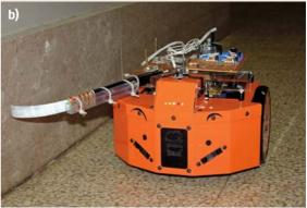
Fig. 60.7 (a) A simple antenna mounted on a Sprawlette robot ©Mark R. Cutkosky, Center for Design Research, Stanford University. (b) A more advanced tactile device ©Noah J. Cowan, Department of Mechanical Engineering, Johns Hopkins University
