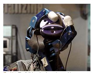
Fig. 28.1 The Salisbury hand grasping an object
