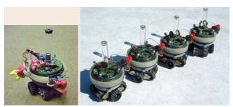
Fig. 61.26 An s-bot and a simulated swarm-bot consisting of four s-bots assembled in chain formation
