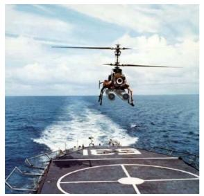
Fig. 44.2 QH-50 DASH unmanned helicopter on final approach (US Navy)
