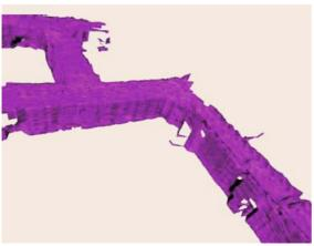
**Fig. 22.17** 3-D indoor map from a swept vertical plane LADAR. Registration is from a horizontal LADAR using SLAM algorithms [22.56]
