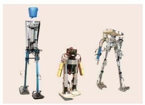
**Fig. 56.10** These robots from Delft, MIT and Cornell (*left* to *right*) are designed to exploit their natural dynamics when walking [56.36]. (Image courtesy of Steven H. Collins)
