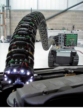
Fig. 11.8 The continuum manipulator (courtesy OC Robotics)
