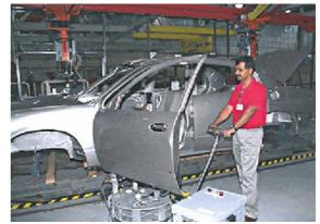
Fig. 57.14 A cobot assisting a human in assembling a car door
