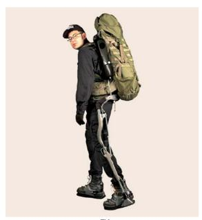
Fig. 33.28 The ExoClimber<sup>TM</sup>field-ready exoskeleton is suitable for rapid ascent of stairs and steep slopes (courtesy of Berkeley Bionics, Oct 2005)
