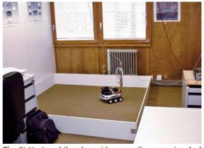
Fig. 61.14 A mobile robot with a pan-tilt camera is asked to move within the walled arena in the office environment
