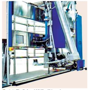
Fig. 3.11 The DeLaval VMS milking robot
