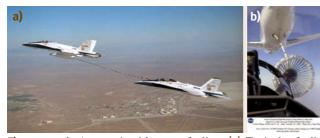
Fig. 44.14a,b Automatic airborne refueling. (a) Typical refueling configuration. (b) Camera view of refueling basket (Source: NASA Dryden Flight Research Center)
