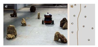
Fig. 36.7 (a) Mobile robot mapping a set of stone rocks. The right image (b) depicts the path and the estimated landmark positions. The manually determined positions of the rocks are marked by *circles* [36.8]
