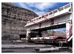
Fig. 49.17 A highwall mining operation
