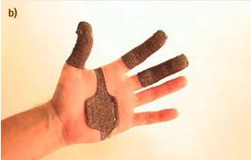
Fig. 4.6 (a) TactArray, a flexible capacitive array tactile sensor from Pressure Profile Systems, Inc., is appropriate for sensing contact locations and areas under sliding conditions. (b) Conformable TactArray sensors can fit on a human or robotic hand (courtesy Pressure Profile Systems, Inc.)
