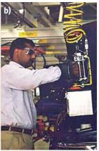
Fig. 33.9a,b The use of IADs for mail and package delivery service (a) and automobile industries (b)
