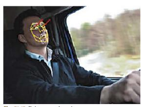
Fig. 51.13 Driver state detection
