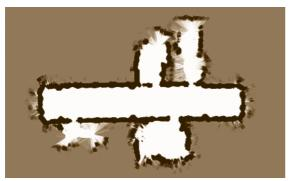
Fig. 36.3 Occupancy grid map obtained from ultrasound data [36.2]
