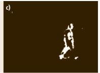
Fig. 22.19a-c Independent motion detection from a moving platform. The reference image (a) is forward-projected using the motion homography to (b); (c) is the difference with the actual image [22.58]
