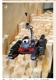
Fig. 50.9a-c View of the NIST standard test bed for search and rescue used by RoboCup Rescue. (a) View of overall test bed, (b) dummy representing a victim, and (c) a step field challenging robot mobility (courtesy NIST)
