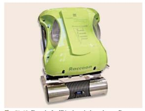
Fig. 54.18 Fraunhofer IPA: the window cleaner Racoon
