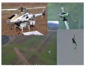
Fig. 44.15 Georgia Tech's unmanned helicopter a parent-child configuration. The child is a hover-capable ducted fan
