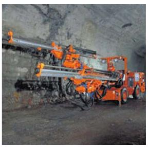
Fig. 49.10 Tamrock drill jumbo for developing tunnels in metalliferous mines
