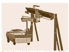
Fig. 57.7 Fanuc's IAD for moving engine blocks [57.53]
