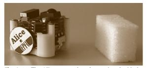
Fig. 61.20 The Alice sugar-cube robot equipped with the evolutionary spiking neural network implemented within its PIC microcontroller
