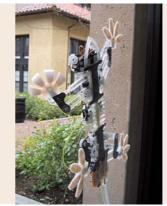
Fig. 60.12 Stickybot, the artificial gecko ©Mark R. Cutkosky, Stanford University Center for Design Research
