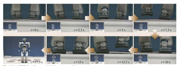
Fig. 56.9 HRP-2 walks on a slightly uneven surface
