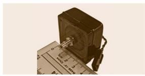
Fig. 3.17 The artificial muscle EPAM motor
