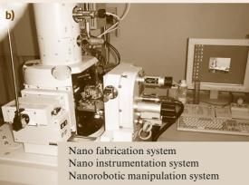
Fig. 18.16a,b Nanorobotic system. (a) Nanorobotic manipulators. (b) System setup
