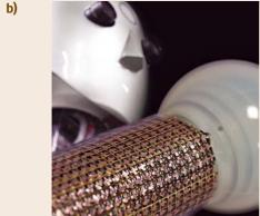
Fig. 60.8a,b Artificial skin devices at Tokyo University. (a) Pressure detection. (b) Pressure and temperature detection © Takao Someya, Quantum-Phase Electronics Center, The University of Tokyo
