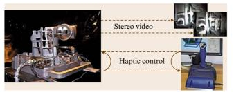
Fig. 31.9 ROKVISS, a telerobotic system providing stereo vision and haptic feedback to the ground operator. (Courtesy of the German Aerospace Center, DLR)
