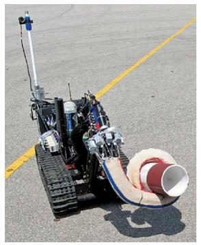
Fig. 60.16 The OCTARM robot ©Ian Walker, Department of Electrical and Computer Engineering, Clemson University
