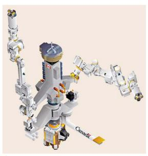
Fig. 11.5 The NASA special-purpose dextrous manipulator (SPDM) (courtesy MDA Federal)
