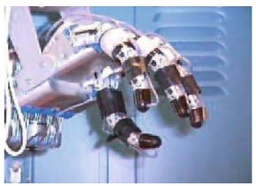
Fig. 15.17 The Utah/MIT robotic hand
