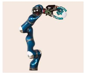
Fig. 57.4 The third version of the DLR lightweight robot (LWR-III) is capable of operating a payload equal to its own weight (13.5 kg)
