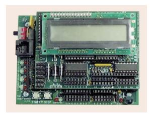
Fig. 55.6 The HandyBoard with its expansion board
