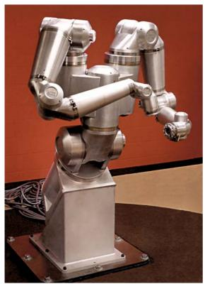
Fig. 11.4 17-DOF robot (courtesy Robotics Research Corporation)
