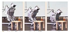
**Fig. 56.32** The humanoid robot H7 executes a motion generated by the autobalancer [56.77]
