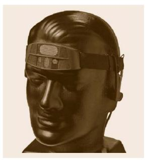
Fig. 21.22 Aid for blind people – the small oval transducer is the transmitter and the other three components are receivers. The large oval receiver provides high resolution, enabling fixation by users' fine neck control (Photo courtesy [21.54])
