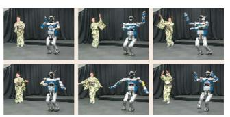
**Fig. 56.3** The humanoid robot HRP-2 dancing with a human [56.22]. The human is a master of a traditional Japanese dance whose dancing was recorded by a motion-capture system, and transformed for use by the robot
