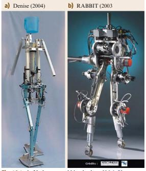
Fig. 16.1a,b Underactuated biped robots [16.1,2]
