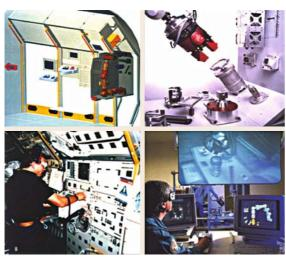
Fig. 45.7 ROTEX manipulator arm onboard the Spacelab D2 mission, the first remotely controlled space robot
