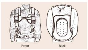
Fig. 33.27 The pilot vests in Fig. 33.10 are designed to distribute the BLEEX-pilot force uniformly on the pilot's upper body
