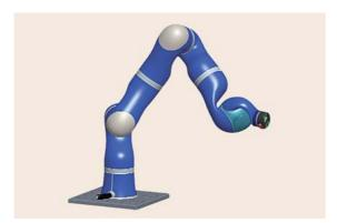
Fig. 11.1 The 7-DOF DLR Lightweight Robot
