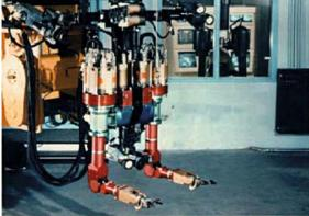
Fig. 48.11 Advanced servomanipulator system (courtesy of Oak Ridge National Laboratory)
