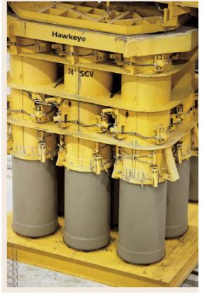
**Table 47.5 (b)** Precast concrete handling robot (courtesy Halo, Inc.)
