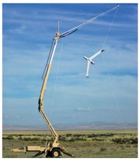
Fig. 44.13 Skyhook system in action (courtesy Insitu, Inc.)
