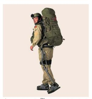
**Fig. 33.25** The ExoHiker<sup>TM</sup> field-ready exoskeleton is suitable for small slopes and can carry a load of 90 kg (courtesy of Berkeley Bionics, Jan 2005)
