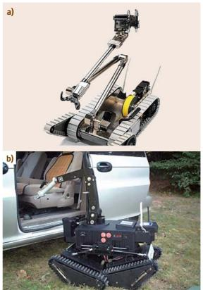
Fig. 48.22a,b Hazardous application robots with manipulator: (a) Packbot with manipulator and (b) Robhaz-dt2 with manipulator
