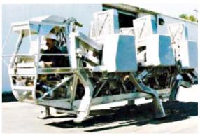
Fig. 16.30 The adaptive suspension vehicle (1986) [16.58]
