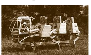
**Fig. 3.3** A photograph of the adaptive suspension vehicle (ASV) walking machine
