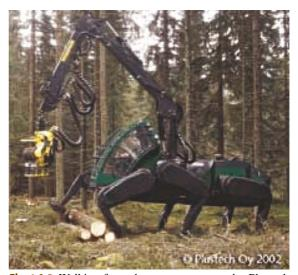
Fig. 46.3 Walking forest harvester prototype by Plustech Ltd., today part of John Deere
