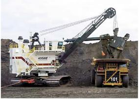
Fig. 49.21 A rope shovel dumping into a haul truck. A truck typically holds between one and three dipper loads of material (©CSIRO)
