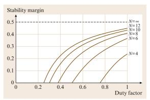
**Fig. 16.29** Optimal wave-gait stability margin of *N*-legged locomotion systems [16.55]
