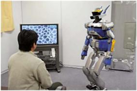
Fig. 56.42 HRP-2 recognizing speech with background noises (TV sound)
