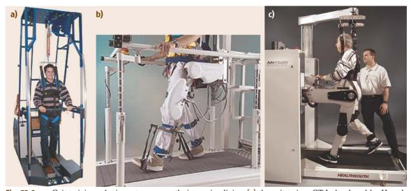
Fig. 53.2a-c Gait-training robotic systems currently in use in clinics; (a) the gait trainer GT-I, developed by Hesse's group and commercialized by Reha-Stim (Germany); (b) the Lokomat<sup>®</sup>, developed by Colombo and colleagues and commercialized by Hocoma AG (Switzerland), and (c) AutoAmbulator<sup>TM</sup>, developed by the HealthSouth Corporation (USA)
