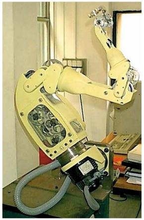
Fig. 13.2 The cable-driven robot *Dexter* by Scienzia Machinale
