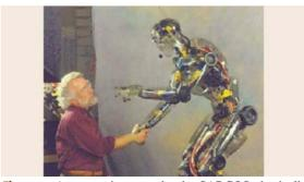
Fig. 57.5 An entertainment robot by SARCOS physically interacting with a bystander. Compliance is built into the actuation system; accuracy and velocity are not primary goals
