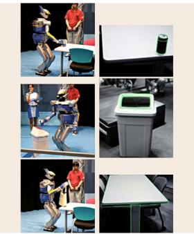
Fig. 56.17 3-D object recognition by HRP-2 using versatile volumetric vision
