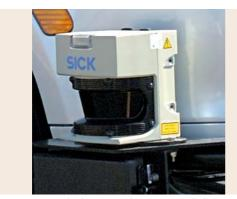
**Fig. 4.8** Example laser ranging sensor (SICK LMS291) that is widely used in mobile robotics
