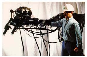
Fig. 33.4 One-handed upper-extremity exoskeleton where a griper allows for grasping of heavy objects [33.21]
