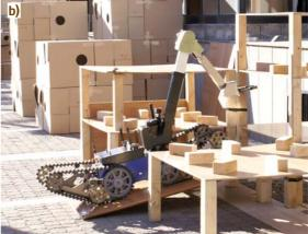
Fig. 50.6a,b Examples of tracked robots with manipulator arms that have been used for disasters or rescue competitions. (a) View from Foster-Miller Talon at the WTC of its arm (courtesy of CRASAR) and (b) telemAX by Telerob at the Rescue Robotics Camp (courtesy of R. Sheh)
