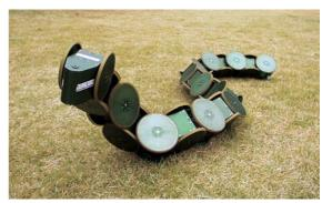
Fig. 11.6 Active cord mechanism (courtesy S. Hirose)
