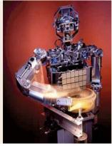
**Fig. 56.20** The humanoid robot Cog used neural oscillators in conjunction with compliant force-controlled arms to perform a variety of everyday tasks with human tools, such as crank turning, hammering, and sawing. Photo by Sam Ogden
