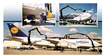
Fig. 3.10 The hydraulic Skywash aircraft cleaning robot
