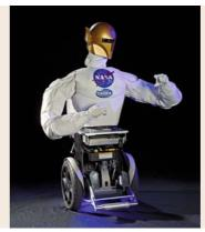
Fig. 56.8 The NASA Robonaut consists of an upper body placed on a wheeled mobile base
