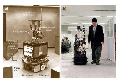
Fig. 55.10a,b The SHAKEY Robot developed in the 60-ties at SRI (a) and the Jijo-2 Robot giving a tour at the National Institute of Advanced Industrial Science and Technology (AIST) (b)
