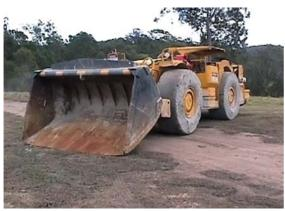
Fig. 49.8 A load haul dump (LHD) vehicle
