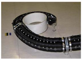
Fig. 11.7 The OctArm continuum manipulator (courtesy I. Walker)
