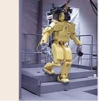
**Fig. 56.2** HRP-1 operating in a mockup of an industrial plant (Courtesy of Mitsubishi Heavy Industries)
