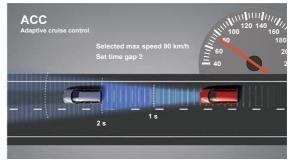
Fig. 51.10 Advanced cruise control (ACC)
