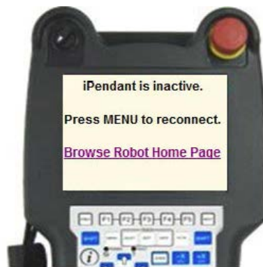
Fig. 13.3.1(c) Disconnected i Pendant screen
