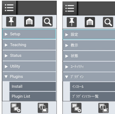
Fig 15.4.3 (a) Pull-down menu displayed when the menu button is tapped (English / Japanese)
